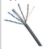
Cat6 has been the enterprise cabling system of choice for many years. Although only designed to run the same Ethernet protocols as Cat5e, it is a higher performance system, supporting more than double the frequency and running to a tighter specification. This gives it significant performance headroom to support the faster protocols like 1000BaseT and is therefore considered more reliable than Cat5e.
